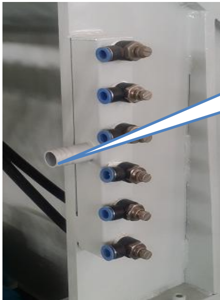
定径套水环体进水口 Water inlet of sizing sleeve water ring body
