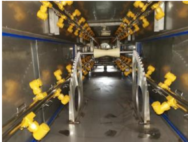
Ø Φ110 ~ Φ450 喷淋箱体中托辊位置 Φ110 ~ Φ450 The position of the roller in the spray box
