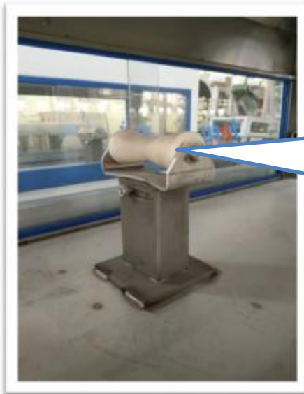
喷淋箱托辊 Spray box roller
